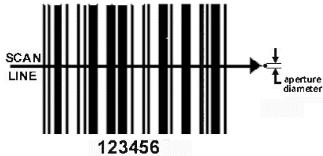
Figure 1 - Scan Line through a Bar Code
